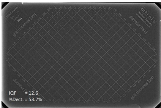
Figure 2 The image of 21 mm breast equivalent phantom using Mo/Mo target/filter
